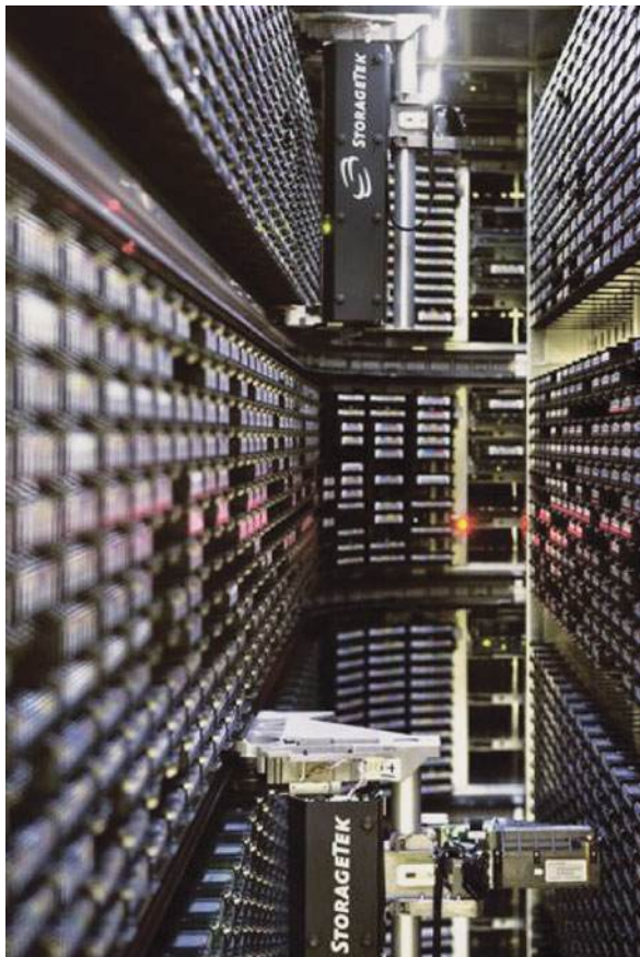
Fig. 2.9 A small portion of the vast, robot-fed magnetic tape storage area that will archive the LHC's "events of interest" data set. (Image courtesy of CERN)
