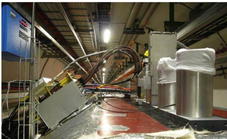
Fig. 7.24 One of the two LHCf detectors, installed along the beam pipe and ready to begin collecting data during the LHC commissioning phase. (Image courtesy of CERN)
