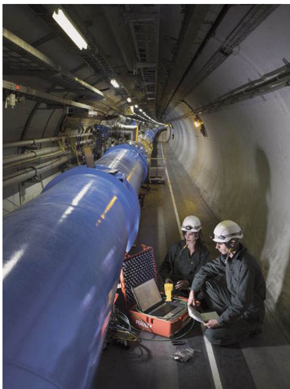
Fig. 2.15 Technicians test one small segment of the 27-km long, super-cooled, cryogenic magnetic proton beam confinement system. (Image courtesy of CERN)
